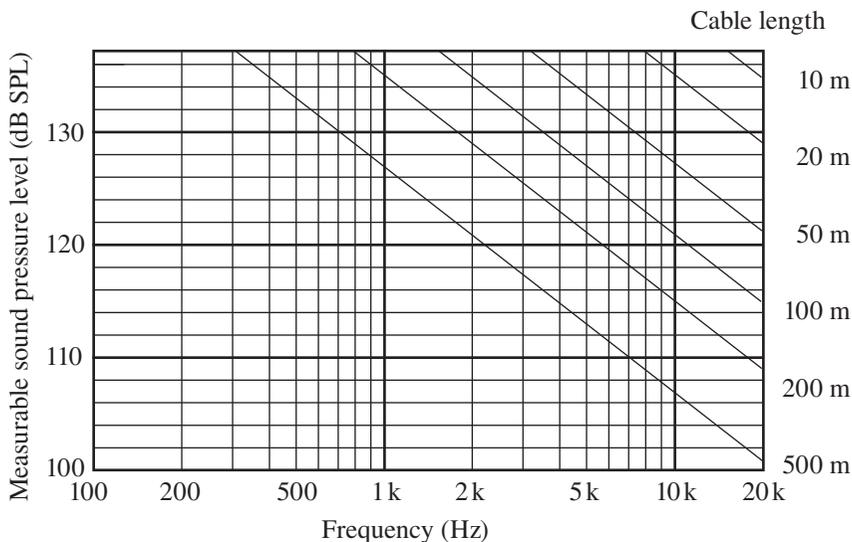
If for example a sound pressure level of 123 dB is to be measured up to 8 kHz, an extension cable length of up to 100 meters can be used.
