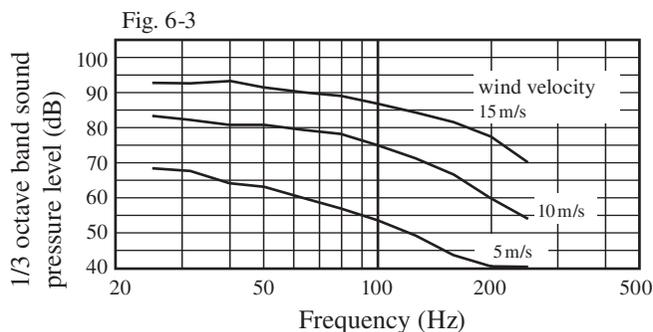
Frequency response of wind noise measured with windscreen WS-10 mounted microphone
