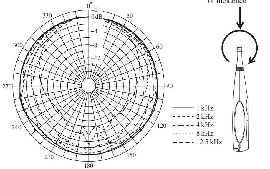
Tab. 1-2 Directional response (Rotated perpendicularly)
