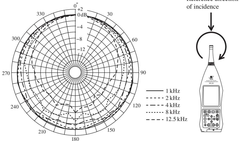
Tab. 1-1 Directional response (Rotated horizontal)
